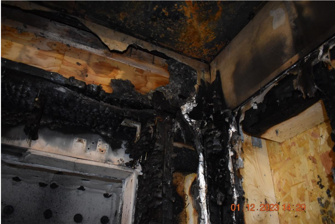
Photo No. 33 Test specimen after the test. Corner below the first flame deflector.
