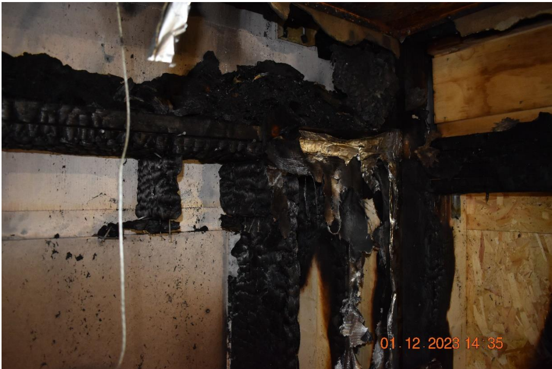
Photo No. 36 Test specimen after the test. Corner below the second flame deflector.
