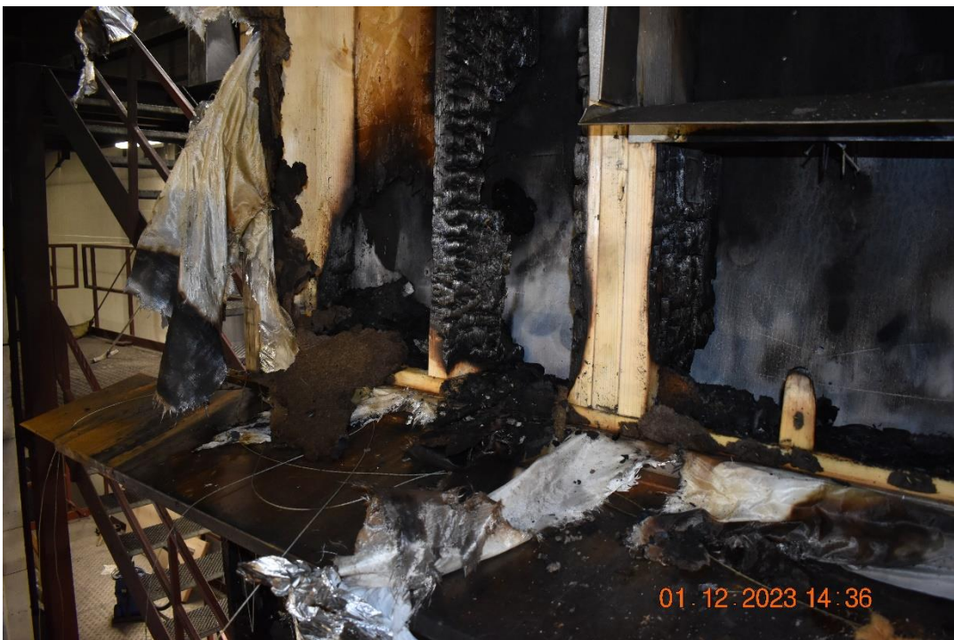
Photo No. 38 Test specimen after the test. Corner below the second flame deflector.
