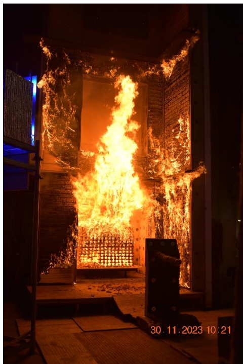
Photo No. 24 Test specimen 21 minutes into the test.
