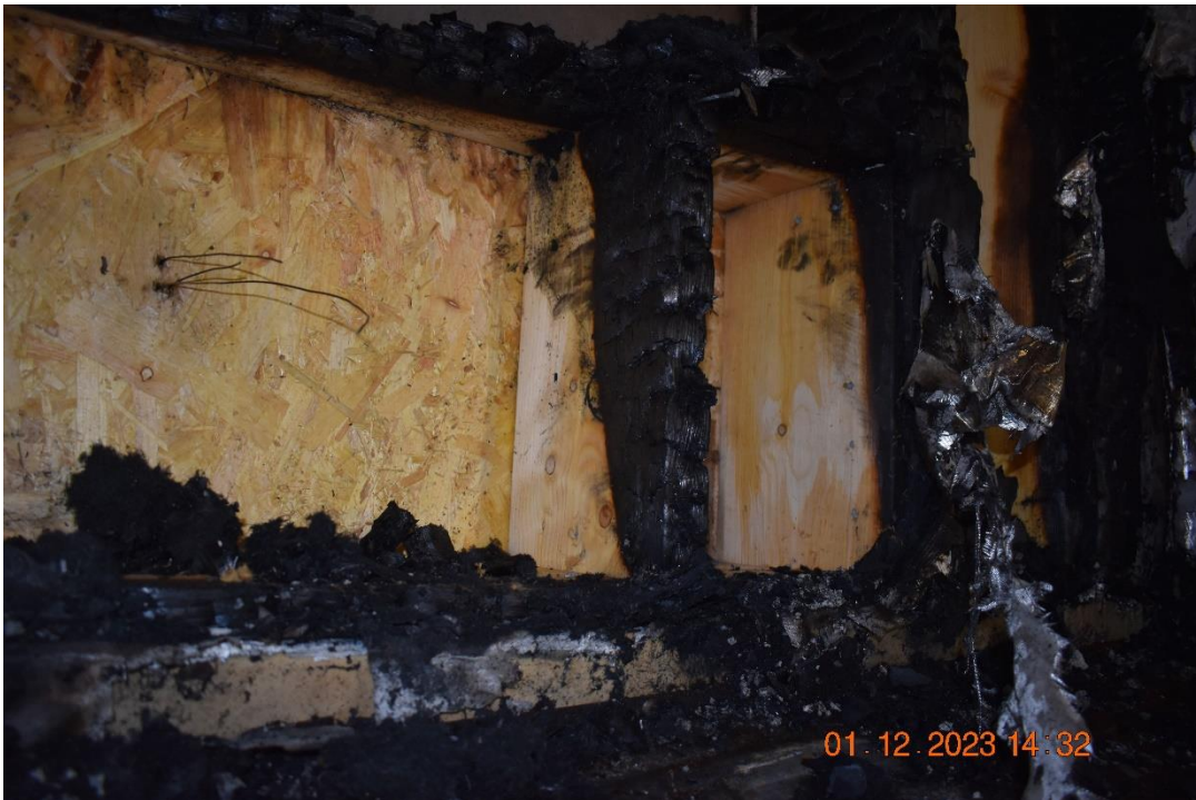
Photo No. 34 Test specimen after the test. Corner above the first flame deflector.
