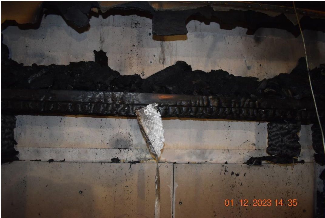
Photo No. 37 Test specimen after the test. Cassette between the first window and second flame deflector.
