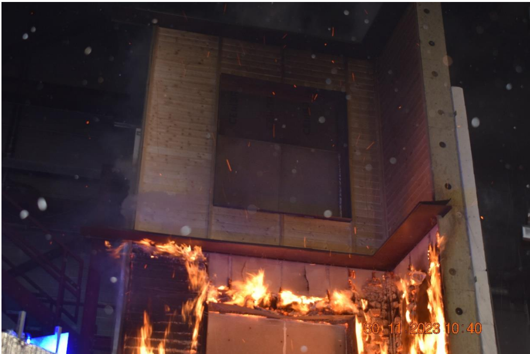
Photo No. 28 Test specimen 40 minutes into the test.
