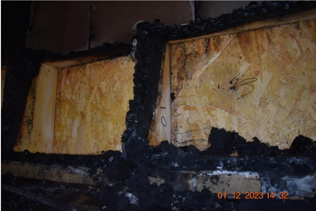
Photo No. 35 Test specimen after the test. Cassette between the fire chamber and the first window.
