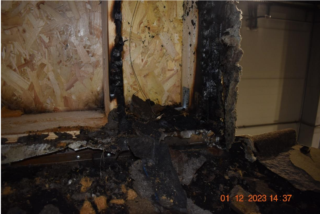
Photo No. 39 Test specimen after the test. Wing façade above the second flame deflector.
